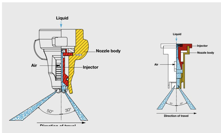
Schematic view of the double flat spray arrangement of IDTA (left) and IDKT air injector twin nozzles.
