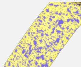
Effect of new nozzle types at increased driving speeds and a water consumption of 150 l/ha each. Trials in Baden-Württemberg, Germany.
